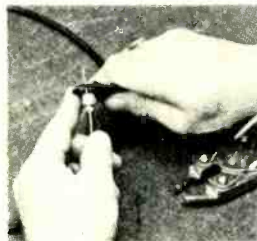
8. Leaving 3/8 inch projecting beyond connector shell, snip off center conductor.
